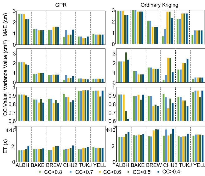
Fig. 6. Comparison of GPR and ordinary kriging for ZWD estimation at six stations by MAE, variance, CC, and ET under different CC thresholds.
