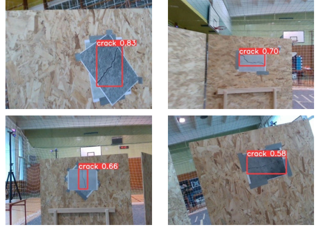
Fig. 18. Crack detection tests with wooden boards background.
